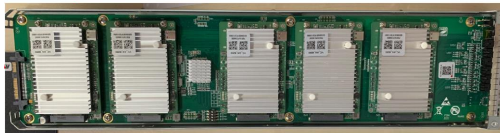
(c) The internal PCB board with 5 SoCs.
