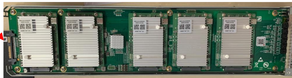
(c) The internal PCB board with 5 SoCs.
