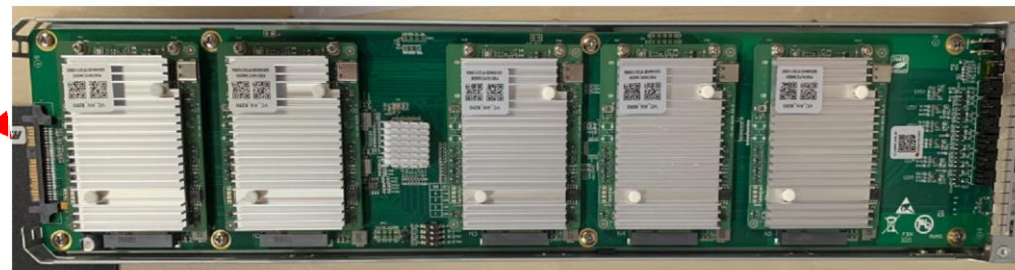
(c) The internal PCB board with 5 SoCs.
