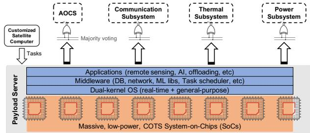
Fig. 1. The proposed satellite architecture for in-space computing.
